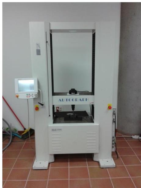
Figura 6.1 Máquina Universal Shimadzu Autograph
