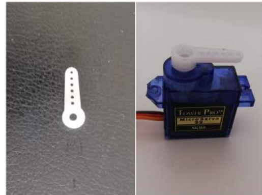
Figure 3.19: Standardized attachment piece used in the micro servo motor.
