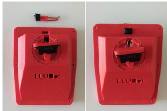
Figure 4.7: Assembly of switch into the hubcap.
