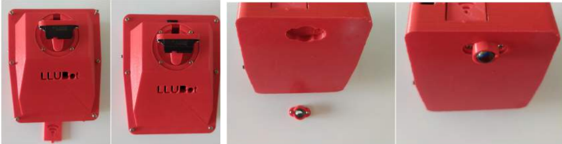
Figure 4.10: Assembly of the chassis, the hubcap and the WiFi cover, as well as the ball caster into the chassis.
