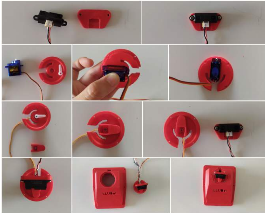
Figure 4.6: Assembly of the fasteners of the sensor's motion system and into the hubcap.
