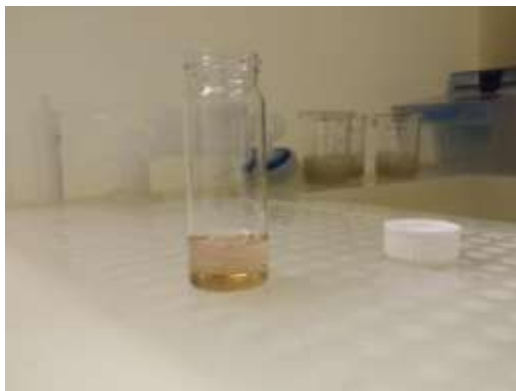
Figure 19. Silver nitrate dissolved in ethylene glycol after an ultrasonic bath.
