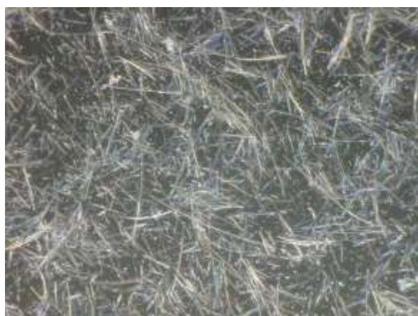
Figure 21. Microscopic picture of the silver nanowire mesh (1000x zoom).
