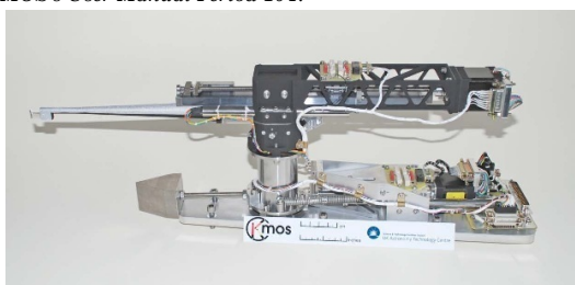
(b) The probe arm based IFU of KMOS. The mechanism is composed of a vertical pivot and an extensible horizontal bar, in one of whose ends there is a pick-off mirror to collect light. Image Credit: KMOS's User Manual Period 104.
