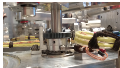
(d) Gear wheel of joint J_2 and the datum switch of the joint.
