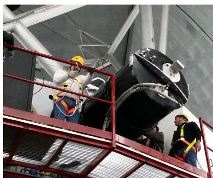
(b) Installation of CIRCE (Edwards et al., 2006; Garner et al., 2016) at one of the four available GTC Folded Cassegrain foci. The cylindrical cryostat of this instrument is similar to the one in MIRADAS. Image Credit: GTC.
