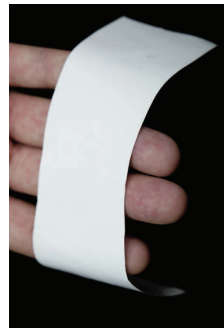
Fig. 4. General view of a green tape of TZ8YS obtained from 45 vol% suspensions. The tape has a 5 cm width.
