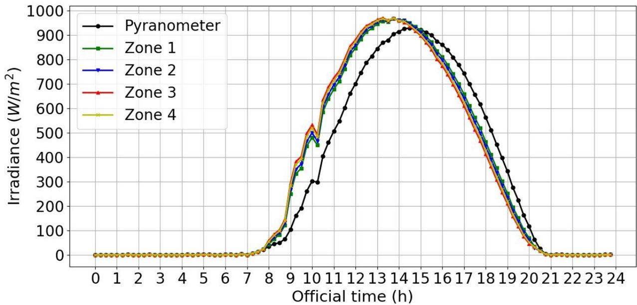
Figure 14: Incident irradiance values measured on the pyranometer and those calculated for each solar carport zones on the 21st of June after the correction factors are applied .
