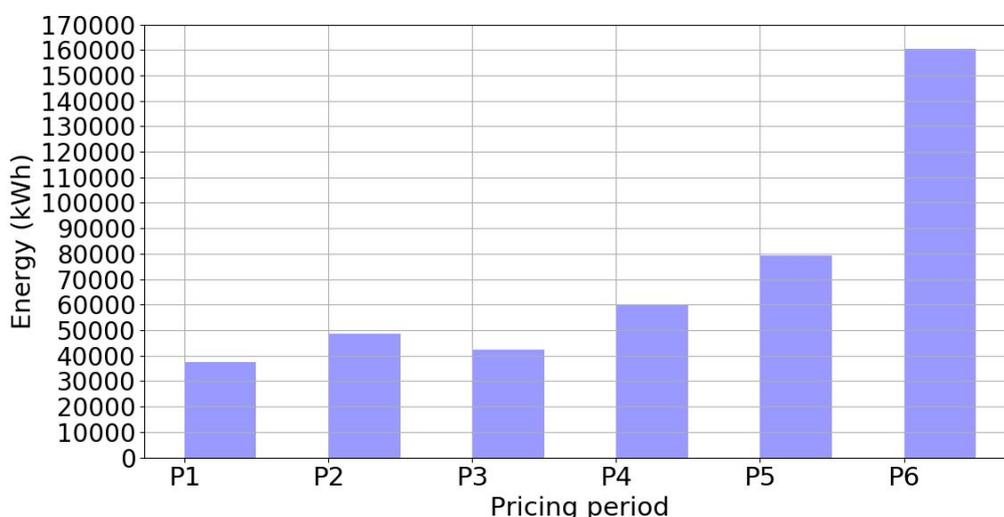
Figure 20: Energy produced by the PV system in each pricing period in the first full year of operation.
