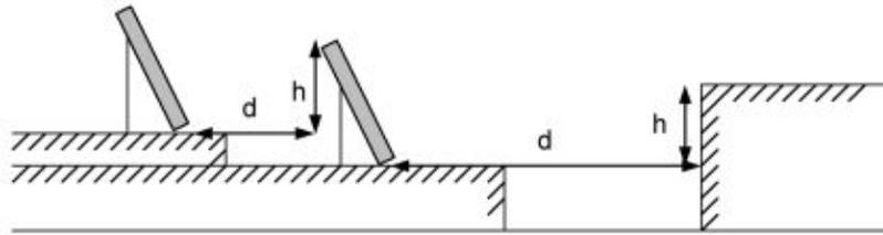
Figure 1: Minimum module inter-row spacing (*d*) for a given height (*h*) [9].
