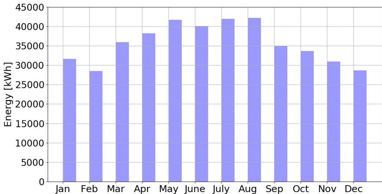
[Figure 17](#): Energy delivered by the PV system in each month of the first full year of operation.
