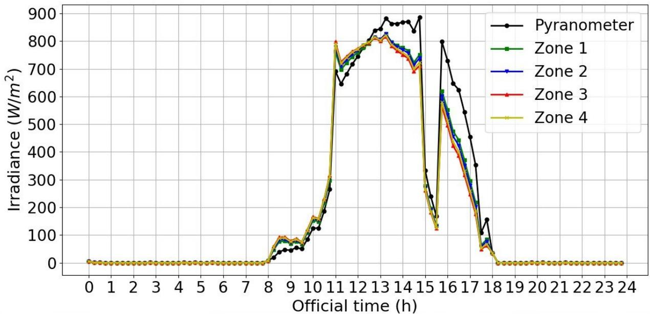
Figure 15: Incident irradiance values measured on the pyranometer and those calculated for each solar carport zones on the 21st of December after the correction factors are applied .
