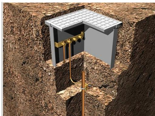
Figure 7: Earthing installation [2].
