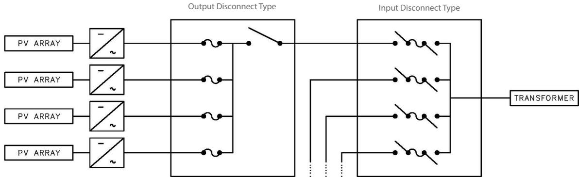
Secondary AC Combiners are typical for sites where further aggregation of AC Combiners is needed.
