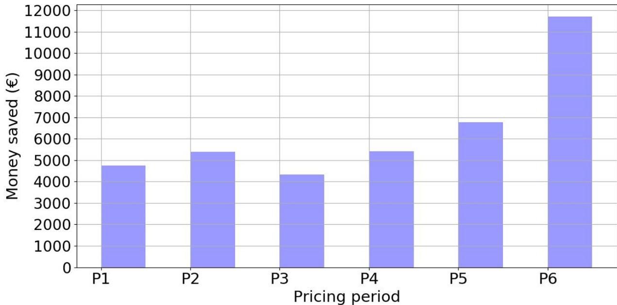
Figure 6: Money saved in each pricing period due to the PV production in the first full year of operation.
