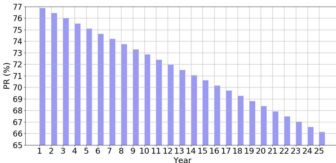
**Figure 18:** Development of the PR of the PV system throughout the years.
