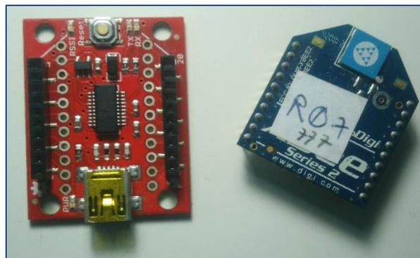
[Fig. 6] Xbee USB Explorer
