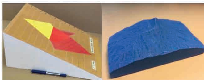
Fig. 3. Left: traditional model with 3D content of land clearance and slope. Right: DTM prepared with 3D printer.
