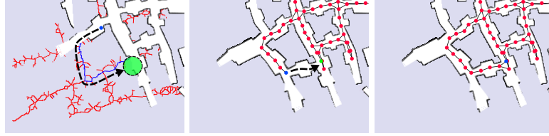
Fig. 5. Illustration of the active loop closing. Left: prediction of the possible path with the loop closure shown in blue. Middle: the robot explores the path along the predicted loop closure and perceives the actual structure of the scene. The graph in the already explored environment shows the pose graph of the SLAM system. Right: successful loop closure. Please note that the predicted environment is actually not identical with the real environment but reveals a similar structure. This similarity resulted in the shown loop closure.
