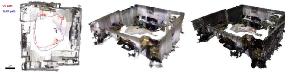
Figure 3.4. Results of the autonomous flight experiment. Left: orthogonal projection of the recovered point cloud map. The path generated by the visual odometry and the corrected SLAM path are shown. Middle: side view of the point cloud map. Right: side view of the octomap.
