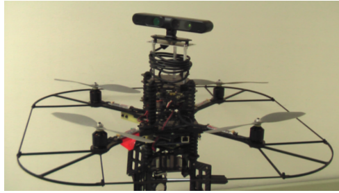
Figure 3.1. The CityFlyer MAV equipped with an Asus Xtion Pro Live RGB-D camera.
