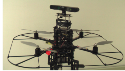
Fig. 1. The CityFlyer MAV equipped with an Asus Xtion Pro Live RGB-D camera.
