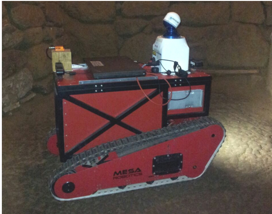
Figure 4.2. A customized Mesa Element threaded robot designed for exploring and digitizing Roman catacombs is the base mobile robot used in this contribution.
