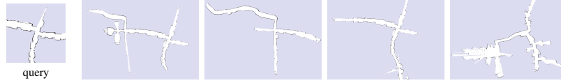
Fig. 3. Example of the submap retrieval using FabMAP2. The left image shows the query map, the other ones the best four matches from the database.
