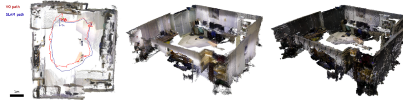
Fig. 8. Results of the real-time onboard SLAM experiment. Left: orthogonal projection of the recovered point cloud map. The path generated by the visual odometry and the corrected SLAM path are shown. Middle: side view of the point cloud map. Right: side view of the octomap.
