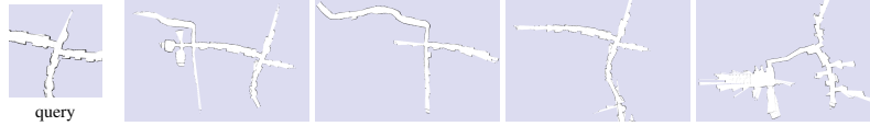
Figure 2: Example of the submap retrieval using FabMAP2. The left image shows the query map, the other ones the best four matches from the database.
