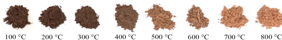
Fig. 15: Color change after controlled burning of sediment from SU XI at different temperatures for 1 h.
