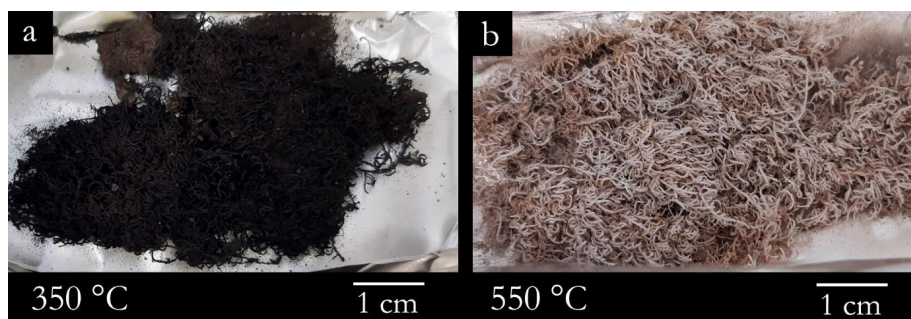
Fig. 21: Moss burnt for micromorphological analysis in the muffle furnace at a) 350 and b) 550 °C.
