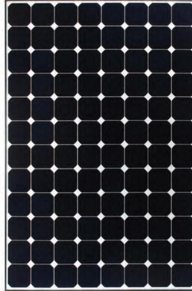
The SunPower™ 300 Solar Panel provides today's highest efficiency and performance. Utilising 96 SunPower all back-contact solar cells, the SunPower 300 delivers a total panel conversion efficiency of 18.4%. The 300 panel's reduced voltage-temperature coefficient and exceptional low-light performance attributes provide outstanding energy delivery per peak power watt.
