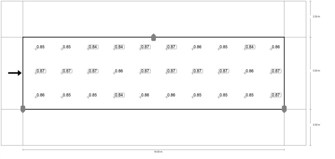
Observer 1: Maintenance value, luminance with dry roadway [cd/m²] (Value grid)
