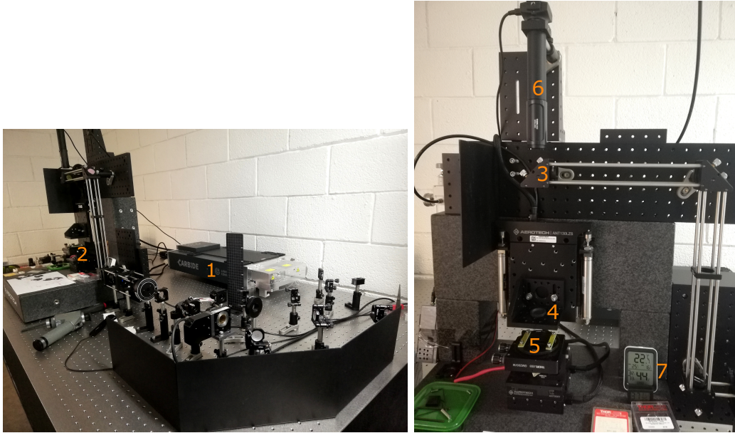
FIGURE 2.1: Experimental setup for the laser inscriptions. Labeled as 1 is the fs laser used, a Carbide model. The laser light is then redirected to the top of the structure to its right labeled as 2. It is then redirected downwards (3) into a lens (4) on an air suspension chamber, which focuses the light onto the sample affixed to the moving platform below it (5). There is also a camera (6) that allows a real-time vision of the sample, as well as a temperature and humidity control device (7).
