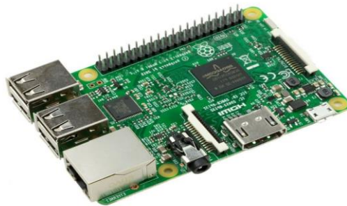
Figura 3.15: Raspberry Pi 3 model B
