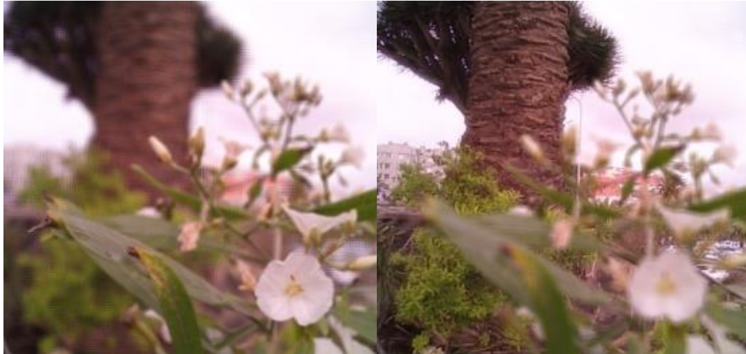
Figure 2. Refocused images from a single shot of a plenoptic camera.
