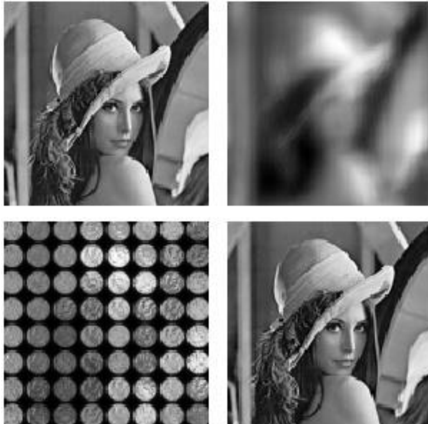
Figure 10. Upper left, original object. Top right, image in the focal plane. Bottom left, image produced by the plenoptic sensor. Lower right, result of deconvolution.
