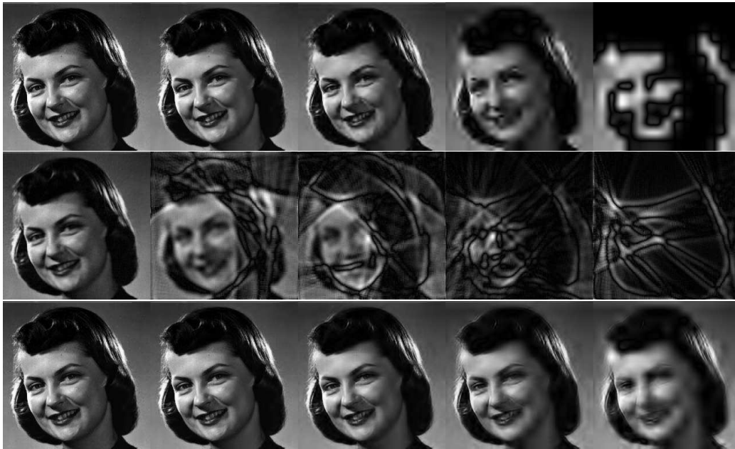
Figure 2.9: Effect of reducing, by hard thresholding, the energy carried by weaker coefficients in different domains, from top row to bottom: Wavelets, Ridgelets and Curvelets. From left column to right: threshold fixed to let pass the 99, 90, 70, 50 and 25 % of accumulated energy.
