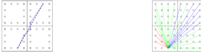
(a) A line in a square of any given scale can be computed by reusing at most three line segments of its 4 children dyadic sub-squares. The discrete lines are not strictly collinear. (b) Number of line segments from 2^{nd} perimeter vertex to each other are represented by a color. Red, green and blue meaning 1, 2 and 3 line segments, respectively.
