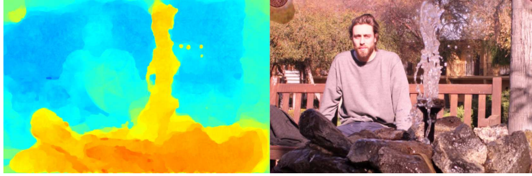
Figure 1.14: Real scene taken and processed in our prototype. On the left, depth-map; right, all-in-focus image.
