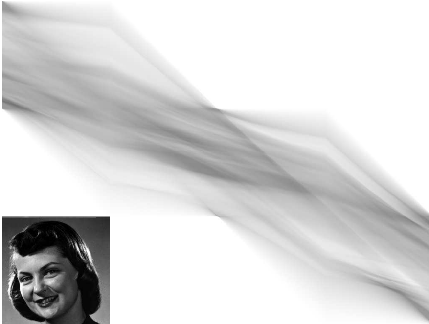
Figure 4.8: A 256 \times 256 gray image, shown on the lower left corner, and its approximate Discrete Radon Transform. Note the increase in size: 6 \cdot N^2 non zero coefficients, in a 3 \times 4 shape the original size.
