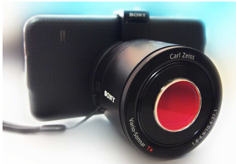
Figure 1.11: Working prototype. The modified Sony QX-100 is attached to a Samsung Galaxy S5 running Android 5.0.
