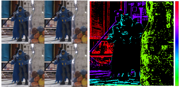
Figure 4.12: Shape-from-focus using aDCT focus estimator applied to a real scene. On the left are shown the four images that constitute the focal stack. On the right, the obtained sparse depth map.
