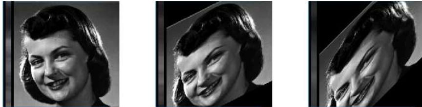
Figure 3.7: From left to right an image sheared to accommodate in a row the discrete lines of Central DRT for minimal, intermediate and maximal slope of the 0 to 45 degrees quadrant.
