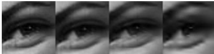
Figure 2.11: From left to right: detail of the eye in the image of example; original detail with simulated defocusing; inverse of Curvelets coefficients carrying 75% of the energy; inverse of Wavelets coefficients carrying 75% of the energy.
