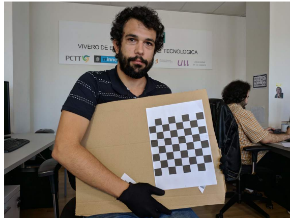
Figure 2.3: Image that contains a printed pattern and can be used to calibrate the camera.
