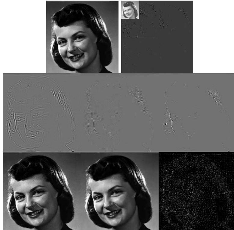
Figure 4.9: A 256 \times 256 image in gray tones on the top left, alongside its decomposition in 3 sub-bands using Wavelets. Middle row, the inversion of exclusively middle and higher Wavelet sub-bands coefficients, and its ratio. Bottom row, the original image and a version of itself where the weakest coefficients on Wavelet domain has been thresholded. On the right it is shown the difference.
