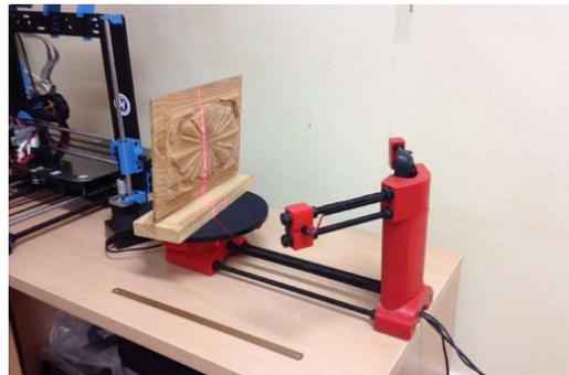
Fig. 5. Scanning process using Ciclop BQ
