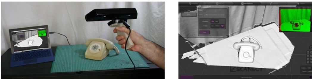
Fig. 1. Scanning process using Kinect Xbox 360 (left) and software Skanect Pro (right)
