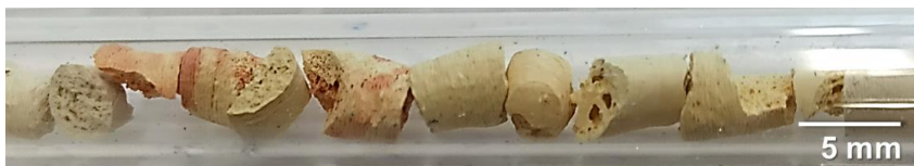
Figure 4.40 Unstructured catalyst devices placed into the reactor tube
