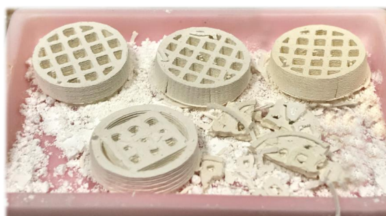
Figure 4. 9 Sintered structures at 900^\circ\text{C} under air atmosphere
