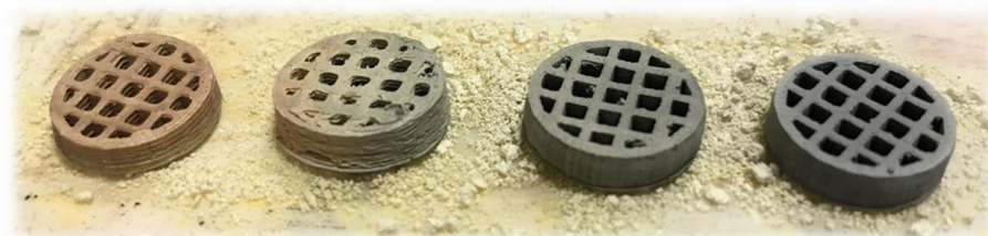
Figure 4. 13 Sintered samples at 1200°C under argon atmosphere (tubular furnace)
