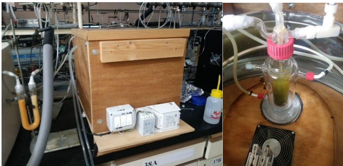
Figure 7 a. (left) Photocatalyst cage, with lamp controllers and the draining system. 10 b (right) Inside the cage
