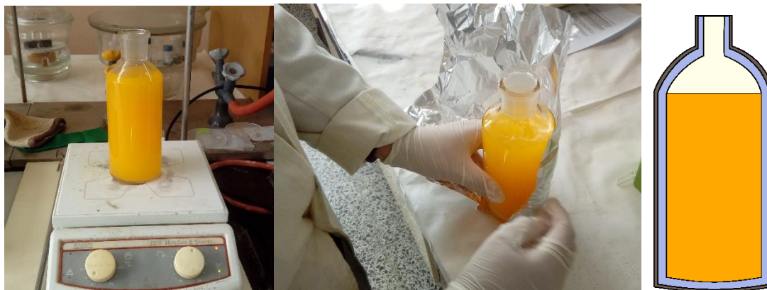
Figure 21. Reactor without jacket. The solution was already poured in. This is before photodeposition.
