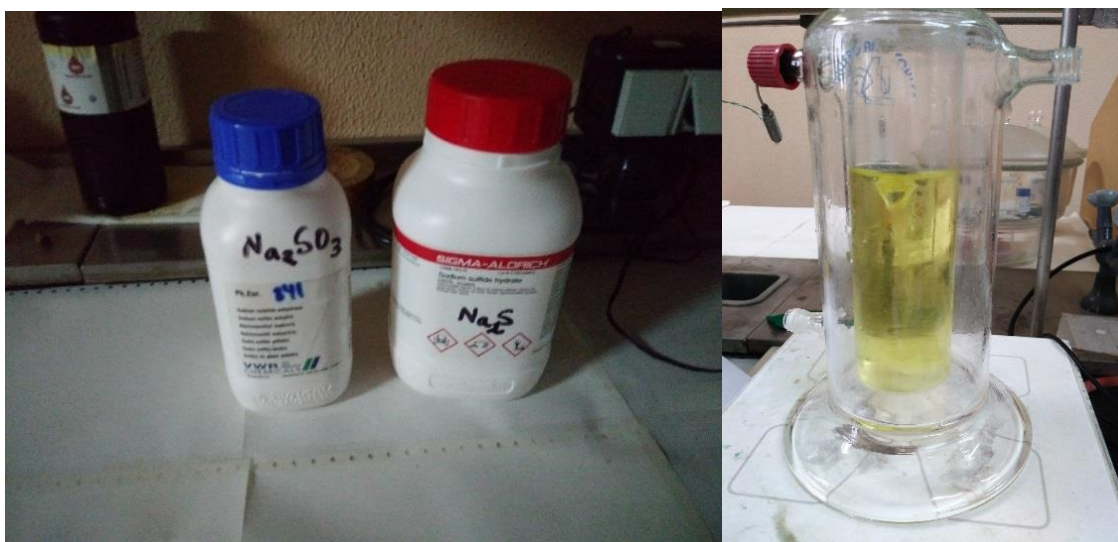
Figure 27 a. (left) Sacrificial reagents. 12 b (right). Reactor after sacrificial reagents are poured. It gets transparent after enough stirring.
