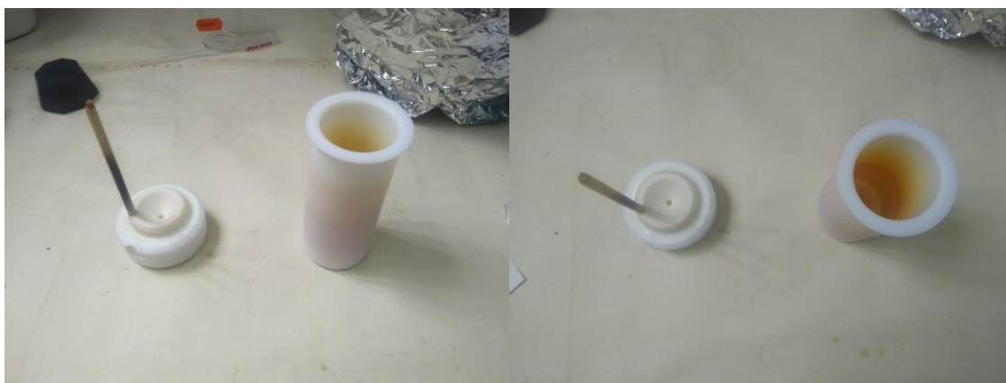
Figure 11. Reactor for the furnace, useful for 60ml of solution. The stick is for temperature control.
