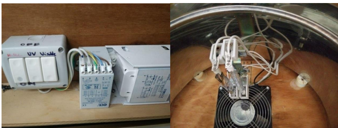
Figure 10 a (left) Detailed of lamp control. 12 b (right) Lamps inside the cage, with a fan for cooling.
