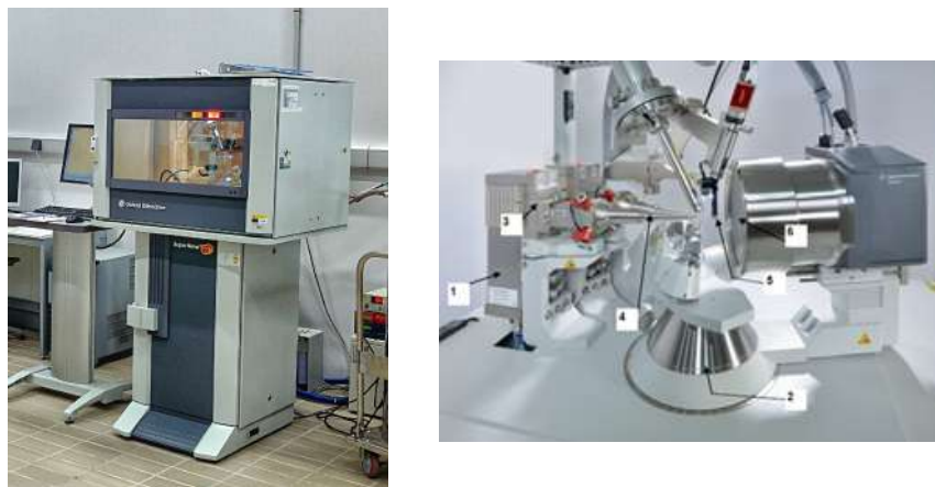
Figure 2.2: SuperNova diffractometer at SEGAI (left) and general view of the X-ray set up (right) with X-ray tube (1), Kappa goniometer (2), X-ray shutter (3), collimator (4), beamstop (5) and Beryllium window (6) [24].
