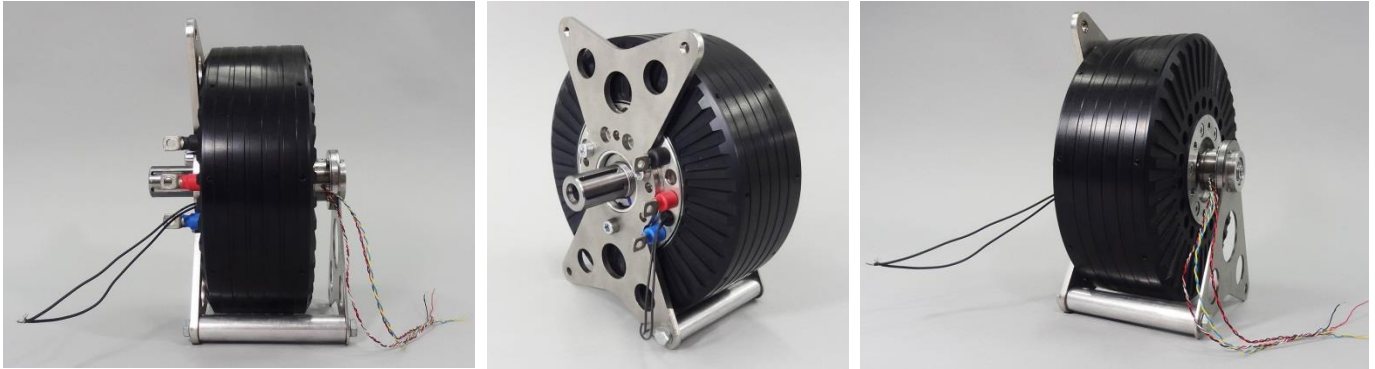
Figure 26: Motor with extended shaft from back motor side
