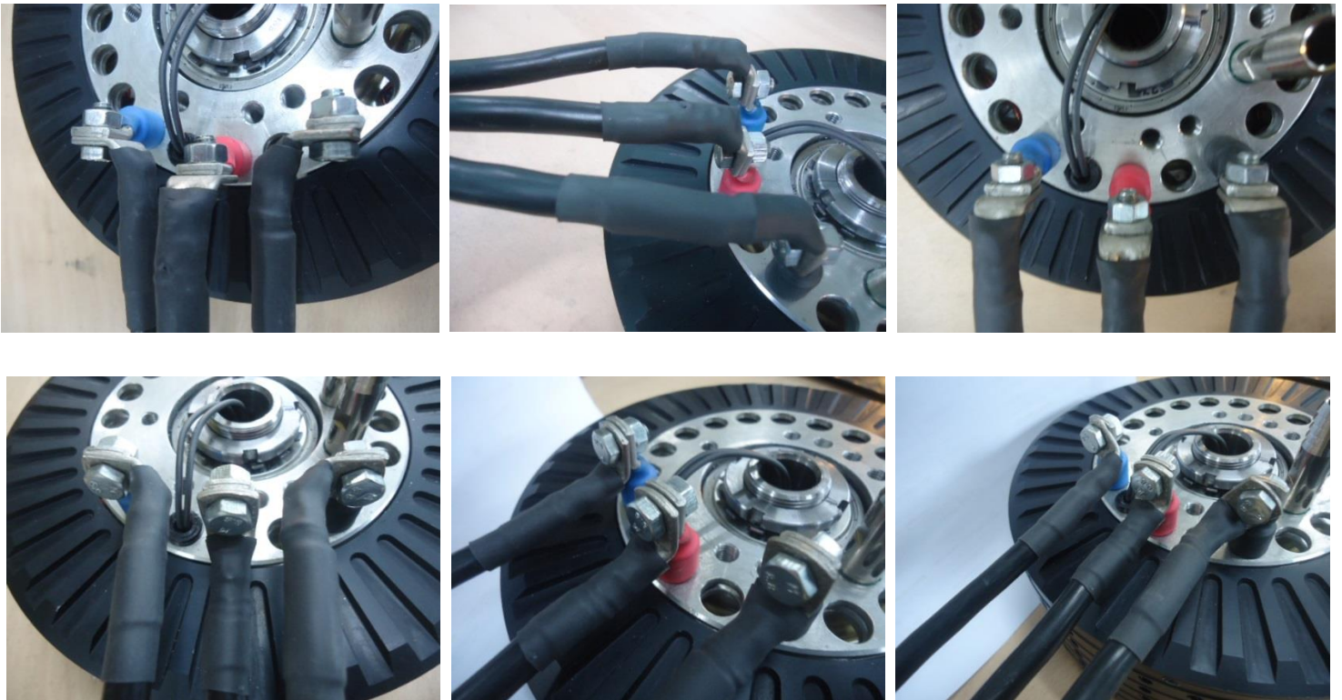
Figure 46: Angular connection of motor connectors to controller cables. Connections must be isolated with shrink hose!
