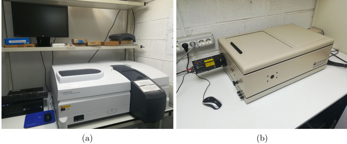
Figura 5: (a) Cary Series UV-Vis-NIR Spectrophotometer; (b) LifeSpec II
