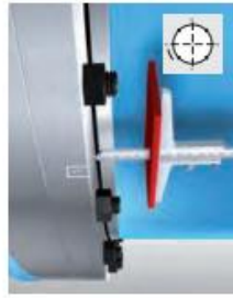
Figure 36: Basic setup for measuring the axial reduction with a depth gauge
