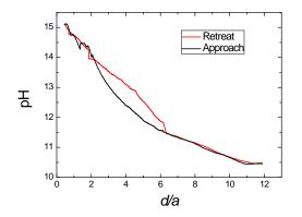
pH distributions above the iron strip measured with the antimony tip as its height was changed relative to the metal surface. The iron-magnesium galvanic pair was immersed in 10 mM NaCl. The direction of the tip movement is indicated in the figures; scan rate: 5 µm/s.
