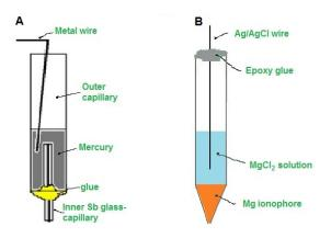
Sketches of the two types of potentiometric tips employed in the SECM measurements: (A) antimony electrode, and (B) micropipette-based Mg<sup>2+</sup>-ISE (containing  $10^{-2}$  M MgCl<sub>2</sub> + 0.25 M KCl as the internal solution).
