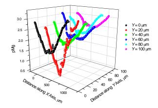
Potentiometric SECM scan lines measured when the tip crossed crossing (X direction) over the magnesium strip in the iron-magnesium galvanic pair immersed in 10 mM NaCl, taken in a plane parallel to the surface of the metal. The different curves were obtained after shifting the tip in the Y direction in 20  $\mu$ m steps. Tip-substrate distance: 75  $\mu$ m; scan rate: 5  $\mu$ m/s.
