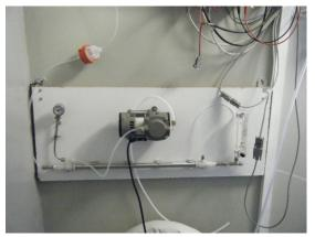
Figure 2.22 Installation of the Nafion dryer for the model 42C-TL at IZO
