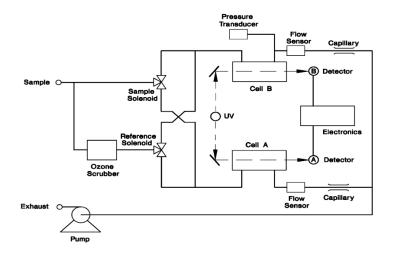
Figure 2.10 Model 49C flow schematic. Source: 49C manual
