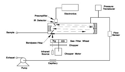
Figure 2.13 Model 48C flow schematic. Source: 48C manual
