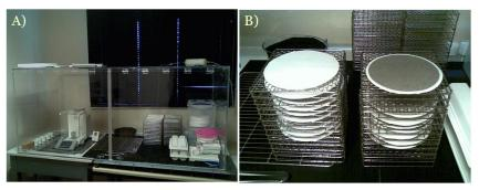
*Figure 2.33* A) Room for preparation and weighting of filters of the CIAI (located in SCO). B) On the left side a blank filter (before sampling), and on the right a filter with a sample of PM<sub>10</sub> particles collected at Santa Cruz de Tenerife are shown
