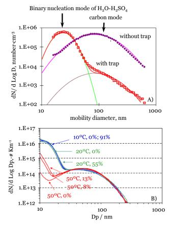
*Figure 1.3.* A) Size distribution of the particles emitted by vehicle exhaust with and without particle trap. Dp: particle diameter. Source: Burtscher, 2005. *B*). Size distribution of the particles emitted by vehicle exhaust under different conditions of temperature and humidity. Source: Casati et al., 2007
