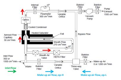
Figure 2.27 Flow schematic of the UCPC (Model 3025 A). Source: user manual
