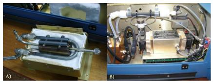
Figure 2.20 Molybdenum and photolytic converters
