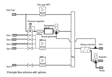
Figure 2.16 MCZ scheme flow. Source: Multigas Calibrator manual
