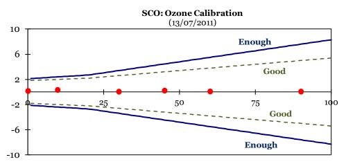
*Figure 2.12* Example of the representation of the response of the analyzer 49C on calibration versus the calibration system (49C-PS). Date: 13/07/2011
