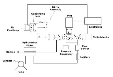
Figure 2.18 Model 43C flow schematic. Source: 43C manual
