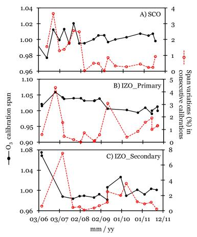
*Figure 2.11* Spans and the corresponding variations of the calibrations carried out to the model 49C at SCO (A) and at IZO (B) primary analyzer and C) secondary analyzer (r<sup>2</sup>>0.99 is found in all cases)
