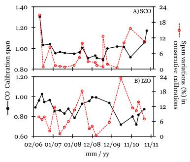
*Figure 2.17* Spans and the corresponding variations of the calibrations carried out to A) the model 48C at SCO (A) and (B) the model 48C-TL at IZO (r<sup>2</sup>>0.9 is found in all cases)
