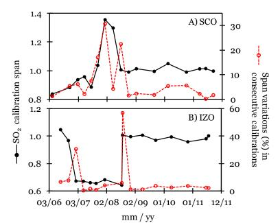
*Figure 2.19* Spans and the corresponding variations of the calibrations carried out to A) the model 43C at SCO (A) and (B) the model 43C-TL at IZO (r<sup>2</sup>>0.9 is found in all cases)
