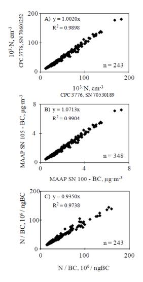
*Figure 2.29* Inter-comparison between the 10 min averaged data recorded with two CPCs model 3776, two MAAPs and the N/BC ratio recorded with these instruments. Data plotted in X-axis were collected with the instruments (CPC SN 70601252, MAAP SN 100) used in this study (Fernández-Camacho et al., 2010)
