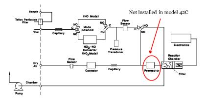
Figure 2.21 Flow Scheme of models 42C and 42C-TL. Source: 42C-TL manuals
