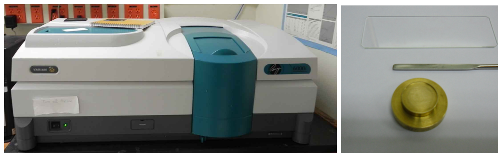
Figure 2.10: Cary 6000i UV-Vis-NIR spectrophotometer (left) and the type of plate used in this instrument (right) in order to obtain the diffuse reflectance spectra of a sample.
