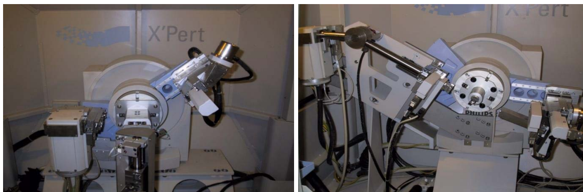
Figure 2.3: Photographies of the diffractometers of the SIDIX at the University of La Laguna: PANalytical X'Pert (left) and PANalytical X'Pert Pro (right).
