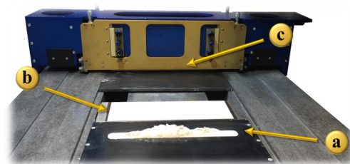
Figure 2. 5 Doctor Blade of the SLA printer a) Paste deposit b) Printing platform c) Blades
