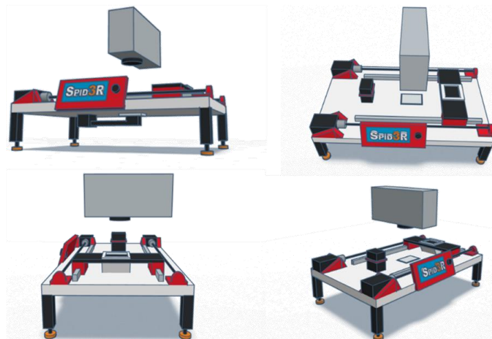
Figure 2. 8 SPID3R, digital design of the DLP prototype printer
