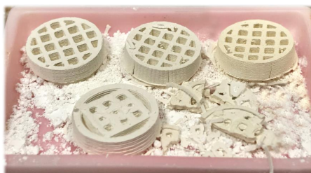
Figure 4. 9 Sintered structures at 900^\circ\text{C} under air atmosphere
