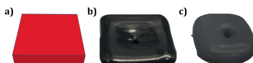
Figure 7. 5 a) Digital square design; b) Fresh printed paste; c) Dried printed paste
