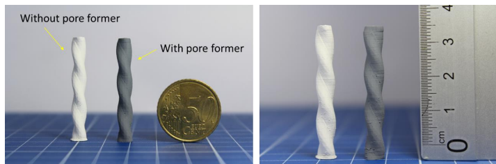
Figure 4. 6 Spiral structures printed by FDM without pore former (white structure) and with pore former (grey)
