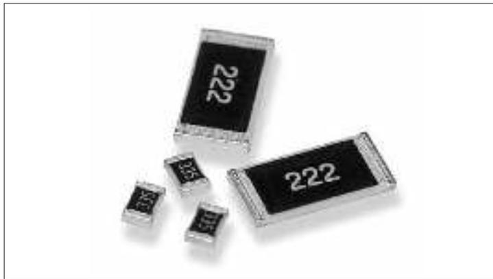
Precious metal terminations are screen printed onto a ceramic base and fired. The resistive element is screen printed and fired and the passivation layer added. Each resistor is trimmed to tolerance by laser. The pre-scribed tile is broken into strips, the end plating is fired on and the strips broken into individual components. Final termination is made by electroplating.
