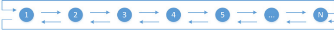
Figure 6: Representation of a 1-D ring communication. Each process sends its data to the next, and receives it from the previous.
