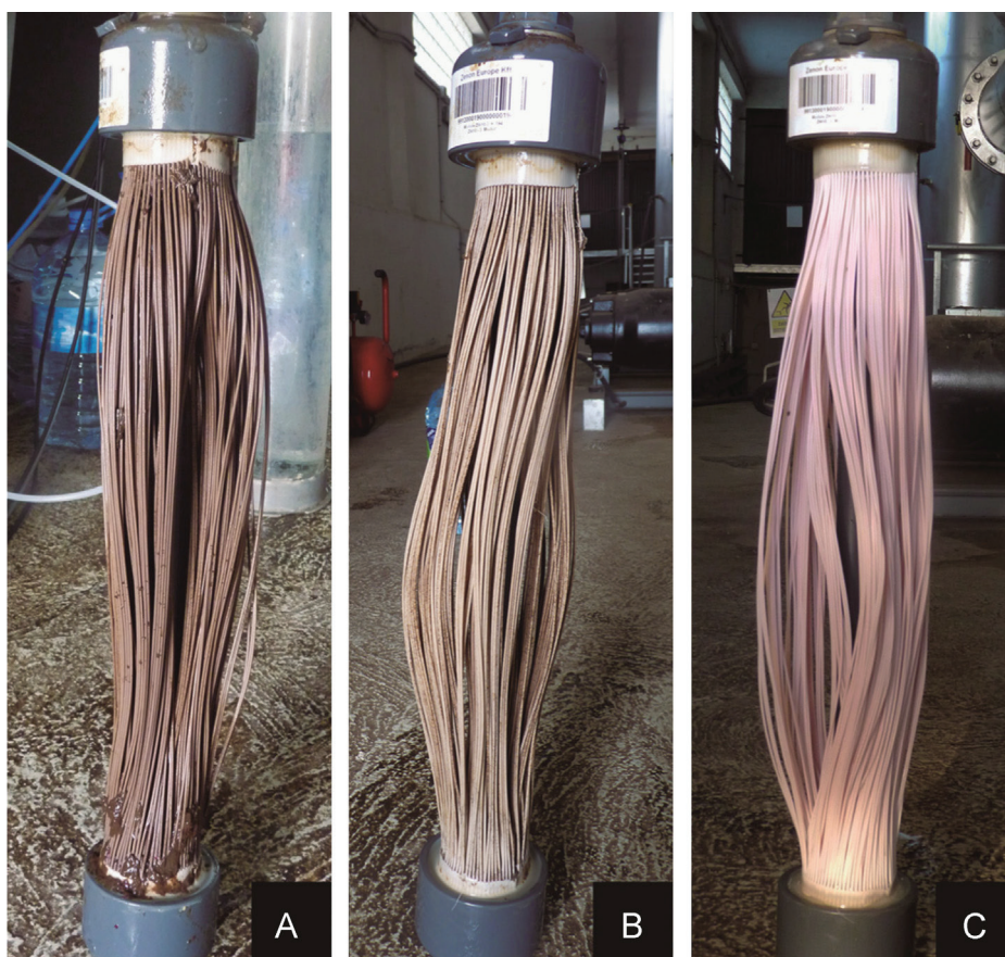
Fig. 10. Membrane before physical cleaning methods (A), after first RC with hypochlorite (B) and finished the cleaned protocol (C).
