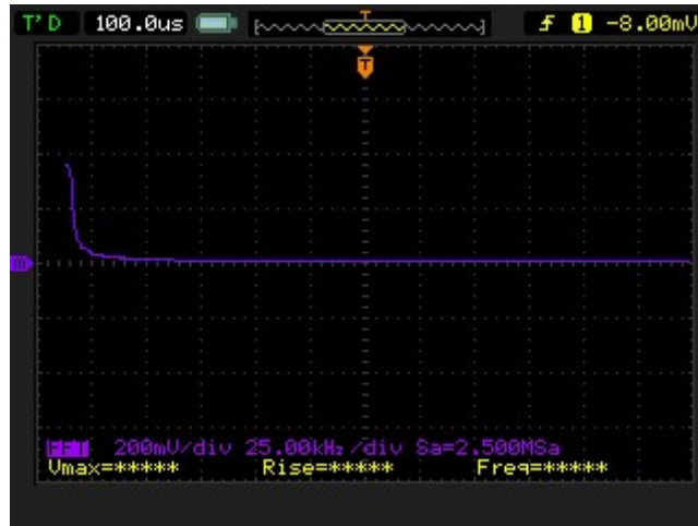
Figura 23. FFT experimental a 1kHz
