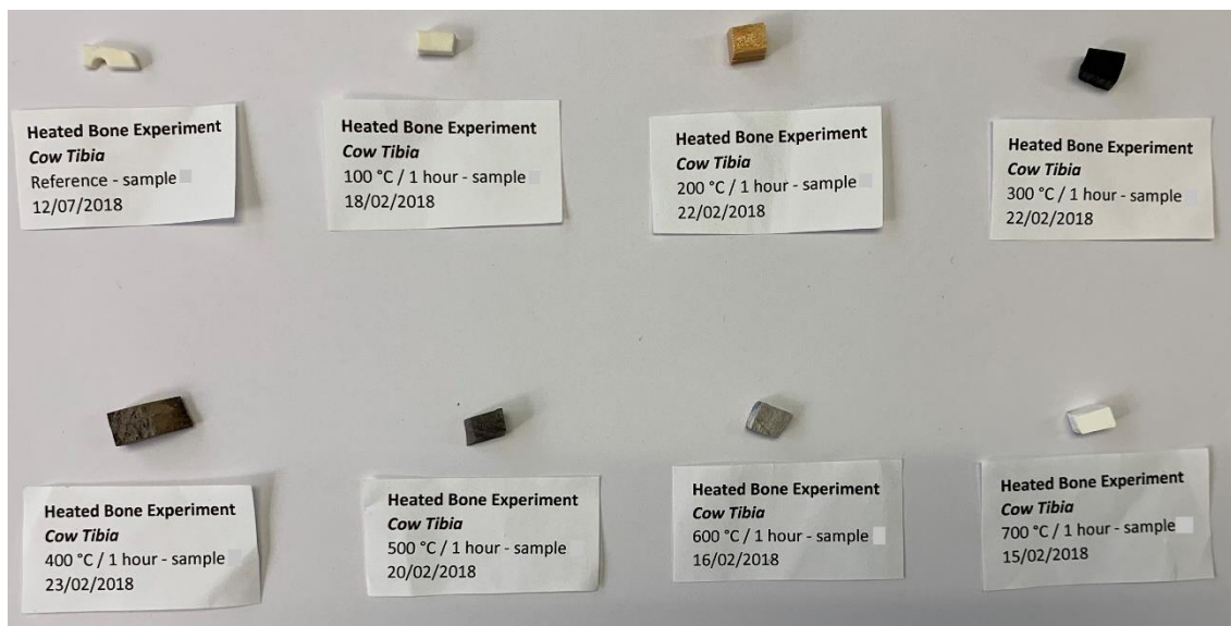
Fig. 3. Cow bone samples without thermal treatment (reference) and heated at different temperatures.
