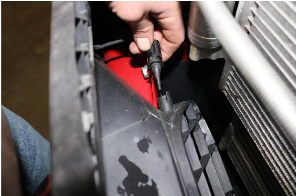
13) Remove the ambient air temperature sensor from it's housing in the front bumper cover.
