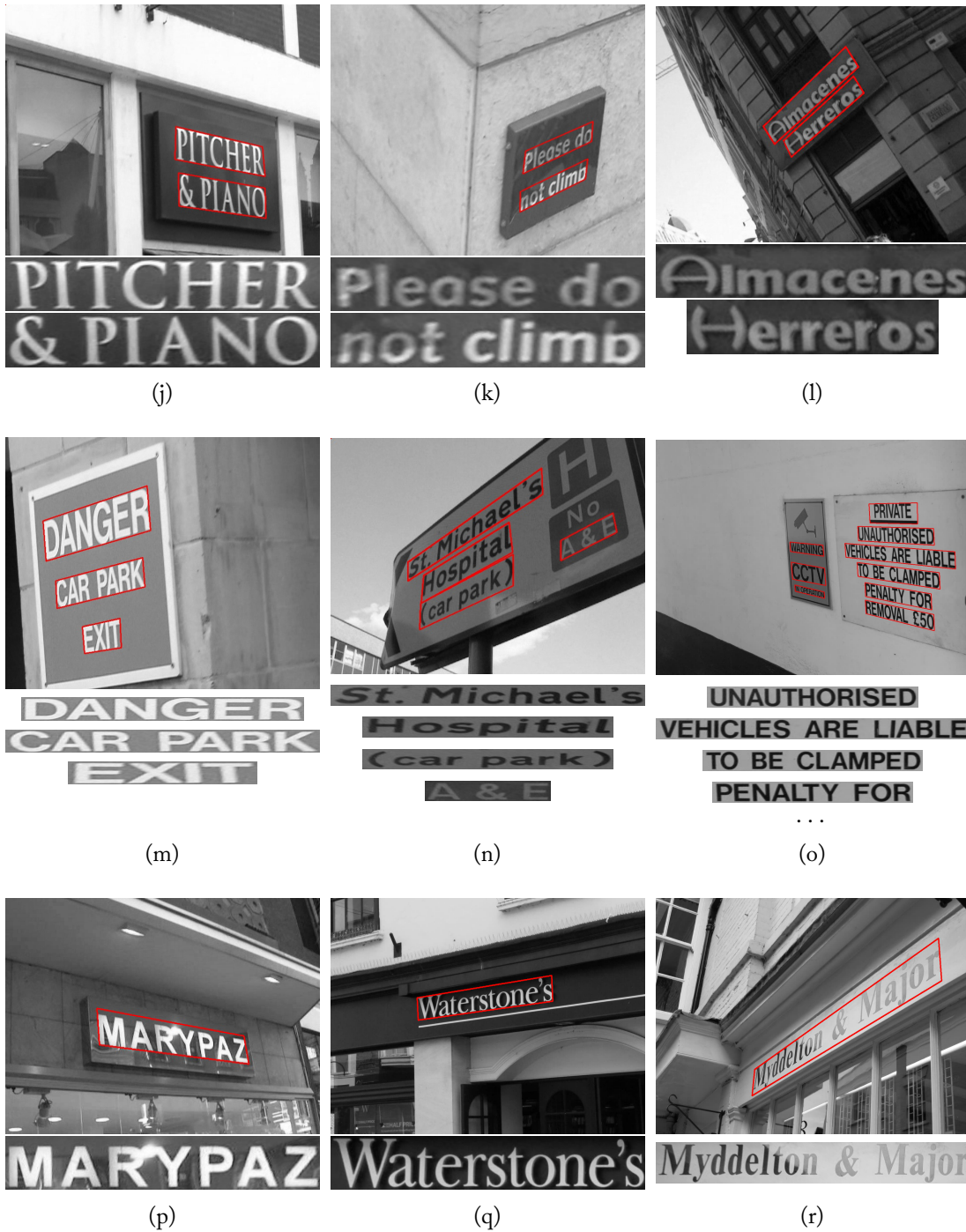
Figure 3.6. A selection of real world images with scene text, along with the text's estimated orientation (red box) and rectified image. ( cont. )
