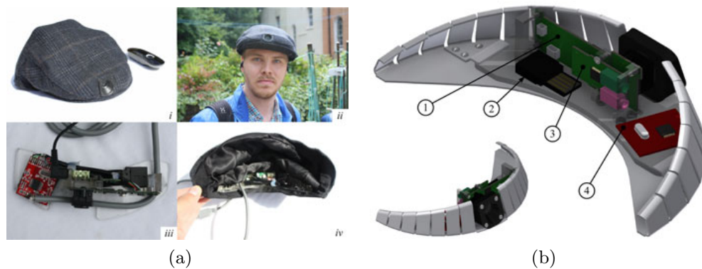
Fig. 1. Developed device together with remote control (a- i ) and its shape when used (a- ii ). Removable part (a- iii ) is placed inside a hat (a- iv ) in a metal framework which is visualized in image (b). The device comprises a USB camera with auto focus (1), a RC receiver (2) and a USB sound card (3) which are connected to a USB hub (4).
