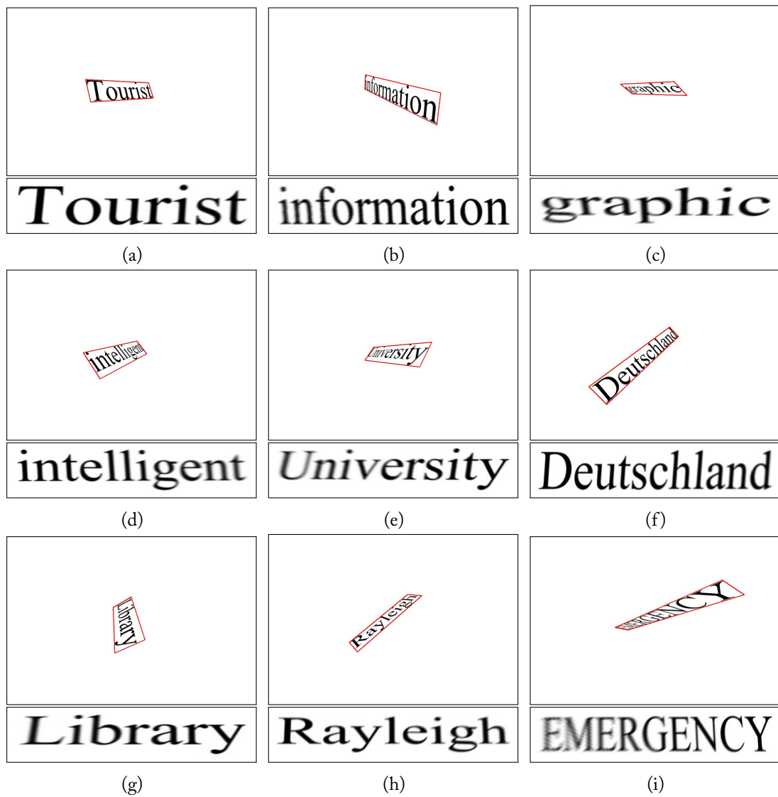
Figure 3.4. A selection of the synthetic images used in the experiments, along with their estimated orientation (red box) and corresponding rectified image.
