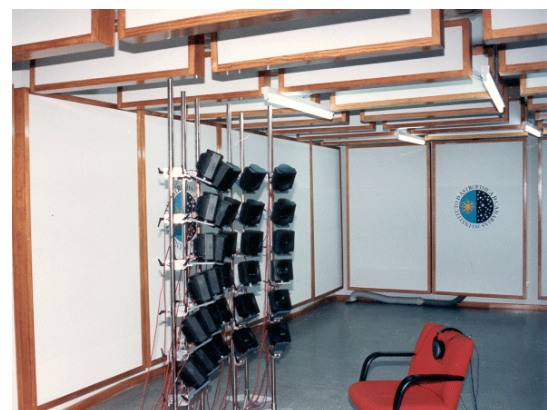
Fig.2. Loudspeakers array inside the acoustically prepared experimental room
