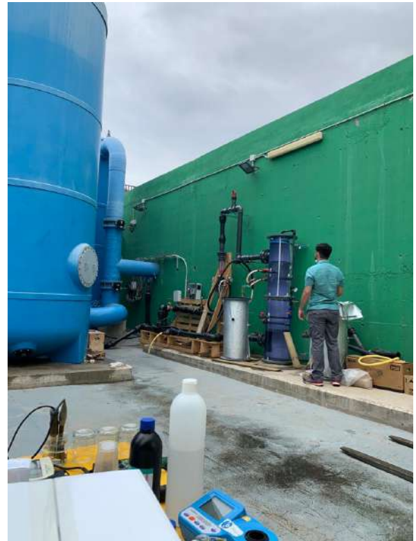
Fig. 1: Experimental set up with transparent CO 2 dissolver. Photo courtesy of Entemanser, S.A., Tenerife, Canary Islands.
