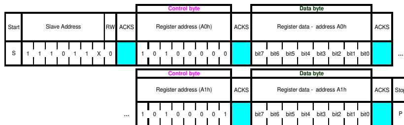
Figure 9: I 2 C multiple byte write (not auto-incremented)
