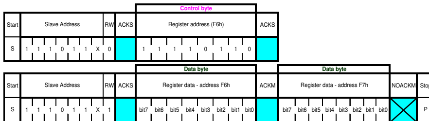
Figure 10: I 2 C multiple byte read
