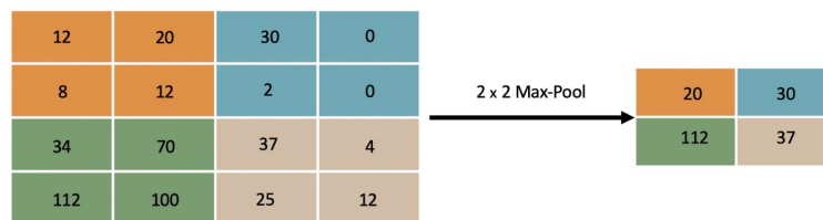
Figure 6: Max pooling layer operation.
