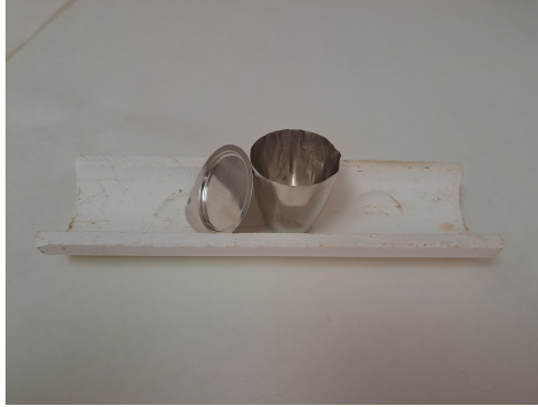
Figure 2.6: Platinum crucible where samples are located to be heated inside the oven.
