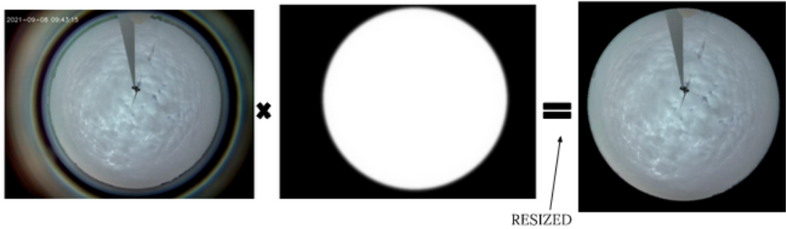
Figure 3.3: Applying the mask and resizing to the original image.
