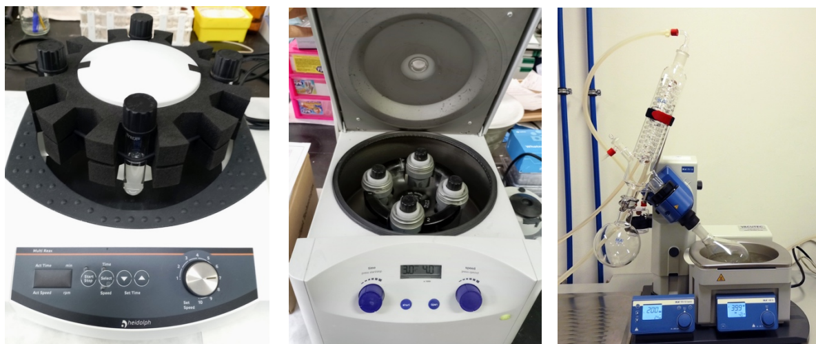
Figure 9. From left to right: Heidolph Multi Reax Top vortex, Eppendorf 5702 centrifuge, and IKA RV10 Rotary evaporator (source: imbm.co ).
