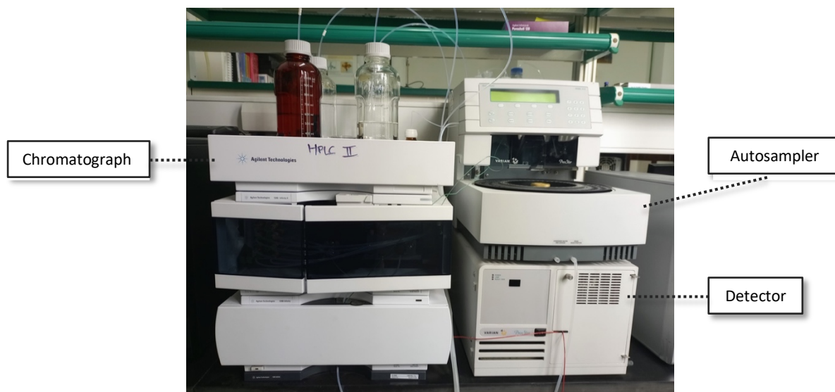
Figure 12. UHPLC 1260 Infinity Series chromatograph, Varian ProStar 410 HPLC Autosampler, and Varian Vis-UV ProStar 325 LC Detector.
