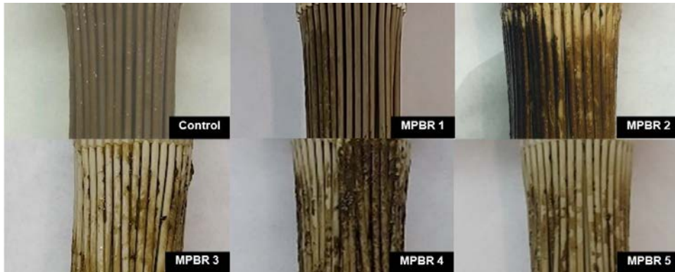
Figure 8. Fouled membranes. Control: HRT=0.75 d, SRT=40 d; MPBR 1: HRT=0.75 d, SRT=20 d; MPBR 2: HRT=0.75 d, SRT=40 d; MPBR 3: HRT=0.75 d, SRT=80 d; MPBR 4: HRT=2 d, SRT=80 d; MPBR 5: HRT=5 d, SRT=80 d.
