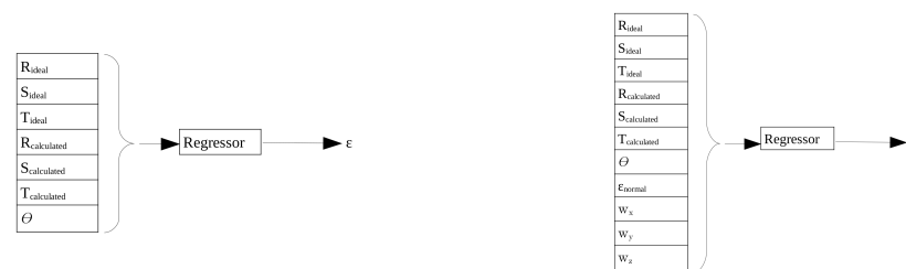
Figure 5. Schematic representation of the information that the regressor receives as input and returns as output (estimated value of \epsilon ). On the left, the inputs are the coefficients of the ideal and calculated planes and \theta value. On the right, four new features have been added as inputs: the coefficients of the axis of rotation between normals and \epsilon_{normal} value.
