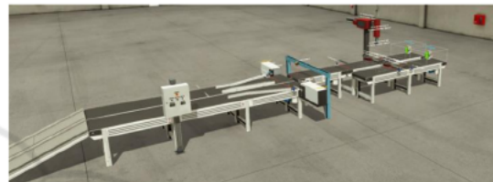
Figure 6: Automation of a parts assembly system and subsequent classification according to the color of the parts.
