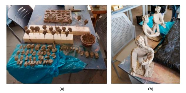
Figure 5. (a) Parts made with the 3D-printed molds. (b) Assembly of the figures using the different parts.
