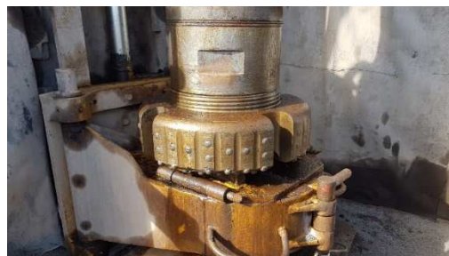
Fig. 5. Drill head with roto-percussion.
