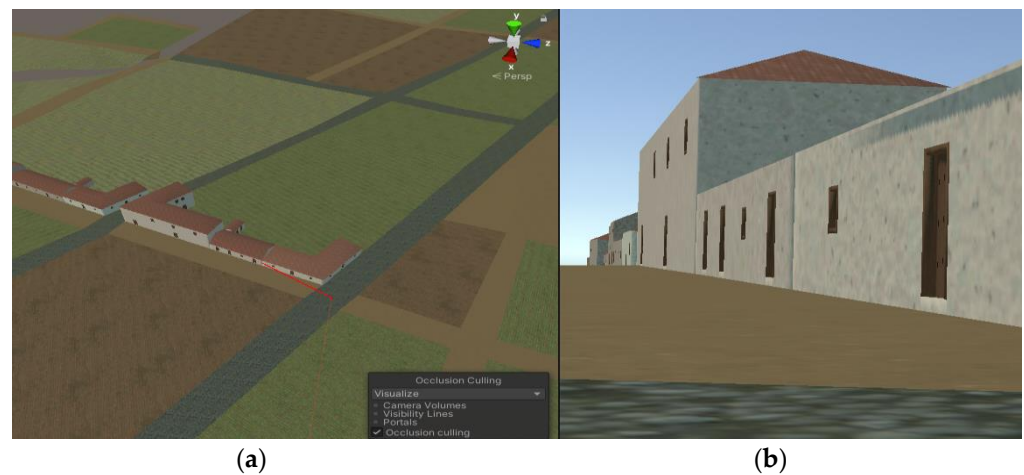
Figure 14. Example of occlusion culling: when looking at the right side of a street (as seen with the red ray in (a)) with buildings on both sides, only the buildings on the side you are looking at are rendered (a). Rendered houses are shown in (b).
