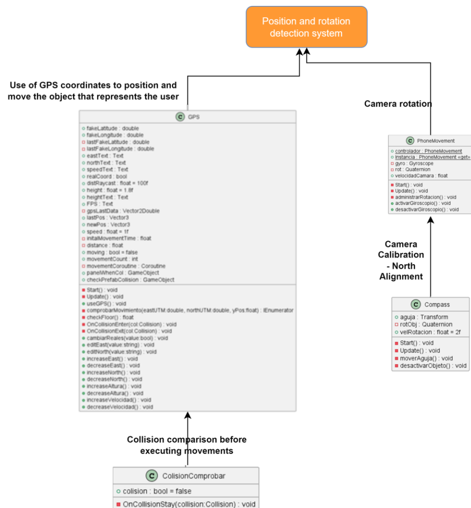
Figure 20. Most important classes in the user positioning and rotation system. (Source: generated by authors).
