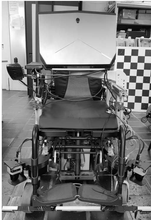
FIGURE 5. Prototype of smart wheelchair implemented
