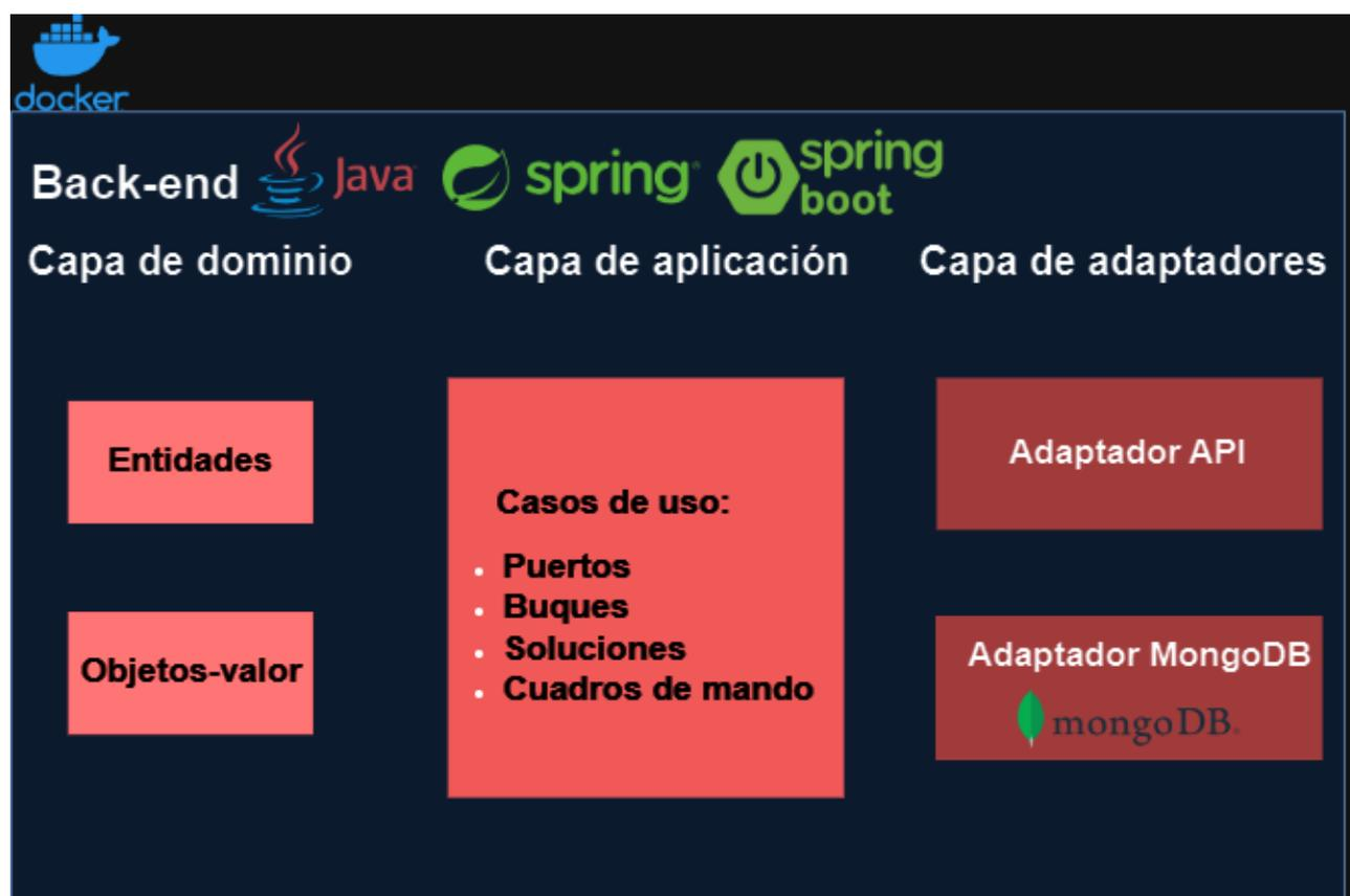
Figura 3.3: Estructura del back-end.
