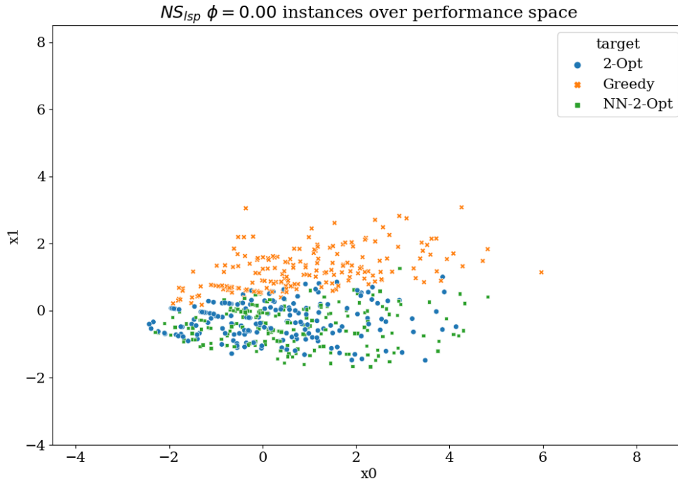
Figure B.1 Instance representation in a 2D space after applying PCAs to all the instances generated by NS_{lsp} setting \phi = 0.0 . The colours and symbols reflect the ‘winning’ solver for each instance. Blue dots are the instances generated for 2-Opt, orange crosses Greedy, and green squares are the instances for NN-2-Opt.
