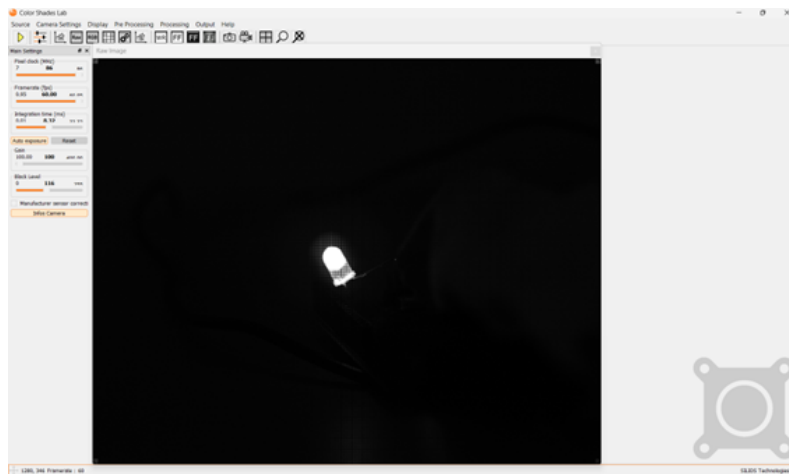
Figure 4.2: Screenshot of the Color Shades Labs software once the multispectral camera is connected and the blue LED is set.
